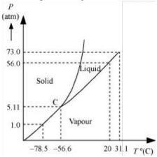
At 1 atm pressure and at  $-60^{\circ}$ C, CO<sub>2</sub> lies to the left of  $-56.6^{\circ}$ C (triple point C). Hence, it lies in the region of vaporous and solid phases.
