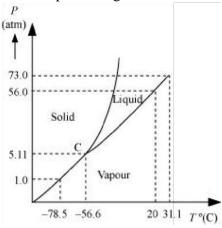
C is the triple point of the  $CO_2$  phase diagram. This means that at the temperature and pressure corresponding to this point (i.e., at  $-56.6^{\circ}$ C and 5.11 atm), the solid, liquid, and vaporous phases of  $CO_2$  co-exist in equilibrium.
