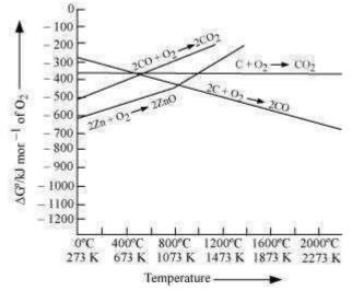
Reduction of ZnO to Zn is usually carried out at 1673 K. From the above figure, it can be observed that above 1073 K, the Gibbs free energy of formation of CO from C and above 1273 K, the Gibbs free energy of formation of CO<sub>2</sub> from C is lesser than the Gibbs free energy of formation of ZnO. Therefore, C can easily reduce ZnO to Zn.
