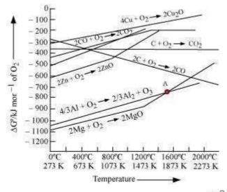
The above figure is a plot of Gibbs energy  ${}^{(\Delta G^{\Theta})}$ vs. T for formation of some oxides. It can be observed from the above graph that a metal can reduce the oxide of other metals, if the standard free energy of formation  ${}^{(\Delta f^{\Theta})}$ of the oxide of the former is more negative than the latter. For example, since  ${}^{\Delta f G^{\Theta}}_{(Al, Al_2, O_3)}$  is more negative than
